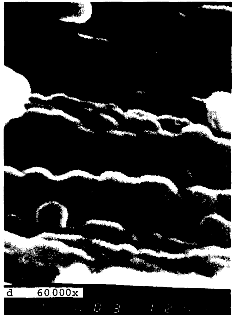
Fig.4. Image of the fracture of a partially reacted calcite monocrystal. Scanning microscopy. Magnification a - 22 x, b - 2000 x, c - 10000 x, d - 60000 x.
